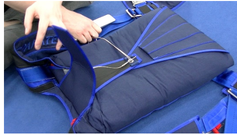
Pic 14.4.3.8 Close flap #6 and use pin of ripcord cable to secure; remove pull up cord and seal pack job
