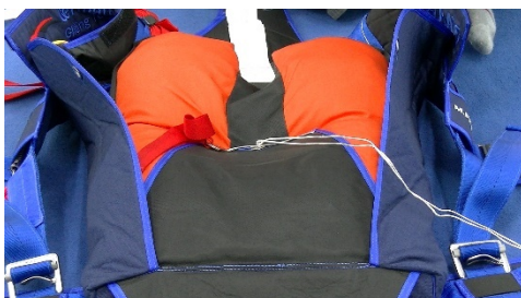
Pic 14.4.2.3 Feed pull up cord through grommet; pull loop up on top of grommet and secure with temporary pin
