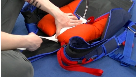
Pic 14.4.2.5 Fold bridle in "S" folds on top of the free bag as shown
