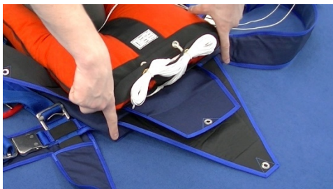
Pic 14.4.2.1 Align corners of free bag to corners of container; Hold down free bag with knee
