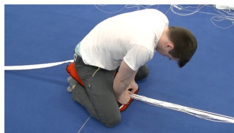
Pic 14.3.3.16 Push all canopy fabric, that is still sticking out of the free bag back in
