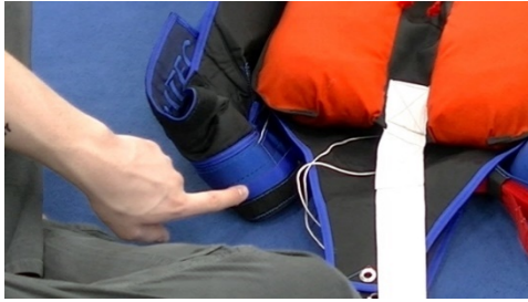
Pic 14.4.1.9 Place risers under the tape to protect them against Velcro wear
