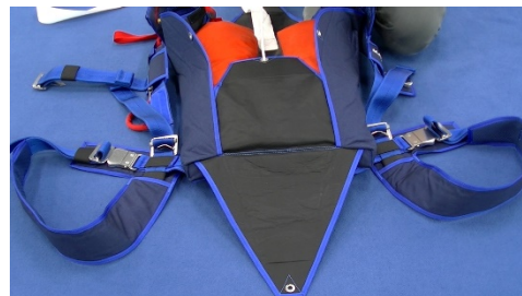
Pic 14.4.2.2 Push corners of free bag into corners of container
