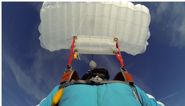
Pic 7.1.1 Flight configuration „Brakes Set”. trailing edge of the canopy pulled slightly down.
