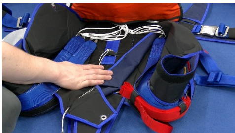
Pic 14.4.1.7 Stow left pair of risers to the side as shown
