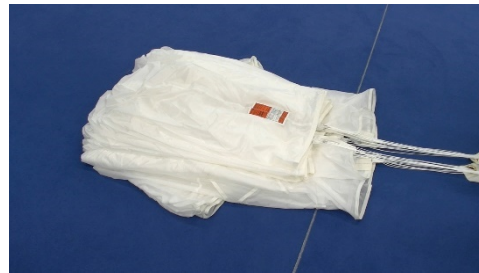
Pic 14.3.3.2 Organized canopy; 3ea. cells left and right; center cell facing down
