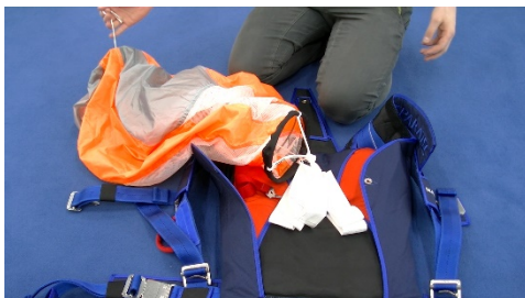
Pic 14.4.3.1 „S“ fold the rest of the bridle in „V“ shape left and right of closing loop, then rout pull up cord through pilot chute from bottom to top
