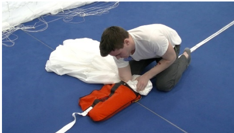
Pic 14.3.3.11 Completely push left side of canopy into left side of free bag
