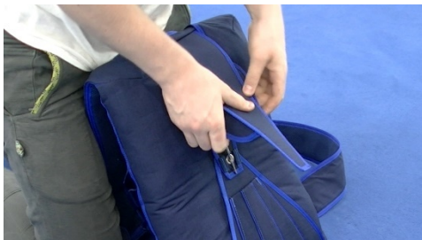
Pic 14.4.3.11 Close top flap and slide in tuck flaps; complete paperwork and put data card behind warning lable on back pad
