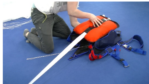
Pic 14.4.1.6 Place free bag gently onto container
