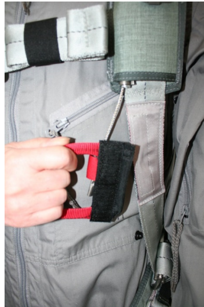
Pic 4.1.2 First pull the handle towards the center of the body , then downwards.
