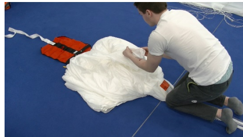
Pic 14.3.3.4 Prepare separation of canopy left and right
