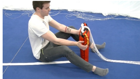
Pic 14.3.3.22 Release the H/C (Pic 14.2.4) Flip the free bag over
