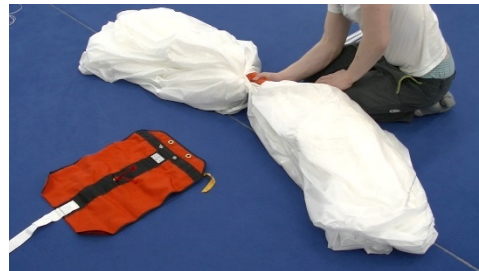
Pic 14.3.3.6 Compress center cell
