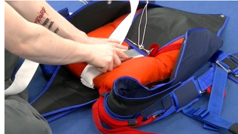
Pic 14.4.2.6 Push the ends of the bridle gently under flap #1 using your tool
