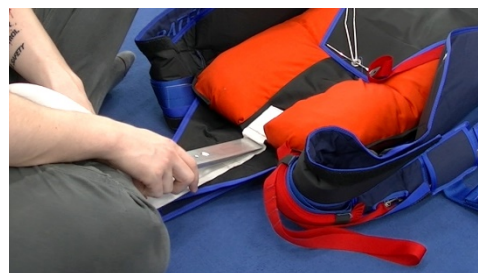
Pic 14.4.2.4 Push first part of the bridle under the free bag using you packing tool
