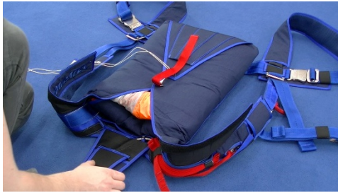
Pic 14.4.3.7 Close flap #5 and compress pilot chute fabric, secure with temporary pin
