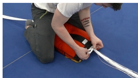
Pic 14.3.3.18 Pull the lines through the elastic; approx. 2 inches
