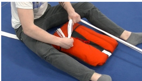
Pic 14.3.3.23 Stow the lines from right to left into the line pouch
