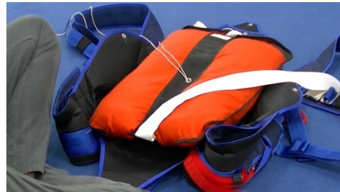
Pic 14.4.1.12 White pull up cord through free bag
