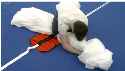
Pic 14.3.3.7 Dress left side of canopy and gently push air out
