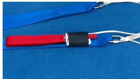
Bild 14.3.1.4 Close the Velcro; make sure to cover up all hook Velcro
