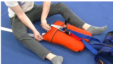
Pic 14.3.3.25 When finished remove Velcro packing aid and match free bag Velcro hook and pile. Do not trap lines doing this
