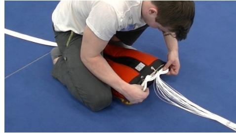
Pic 14.3.3.20 Pull the lines through the elastic; approx. 2 inches
