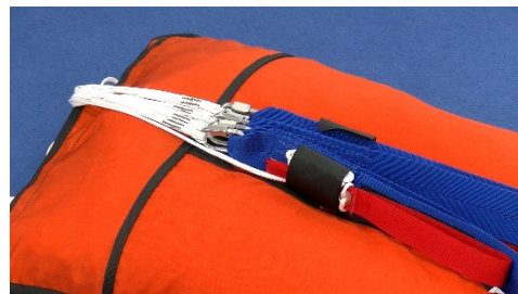
Pic 14.3.3.26 Lines completely stowed and line pouch closed
