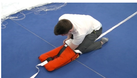
Pic 14.3.3.15 Completely push right side of canopy into right side of free bag
