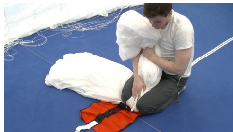
Pic 14.3.3.8 lift up left side of the canopy; cell openings should face down
