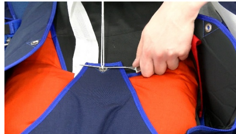
Bild 14.4.2.8 Close flap # 2 (Obere Klappe) and secure with temporary pin
