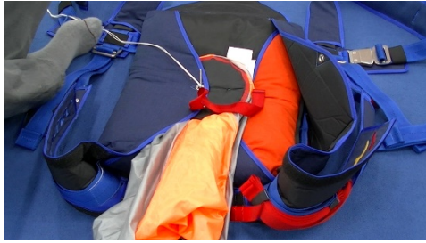
Pic 14.4.3.5 Close flap #3 and secure with temporary pin
