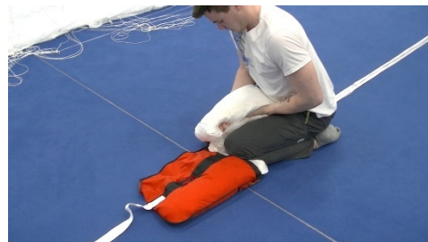
Pic 14.3.3.14 And compress before pushing into the free bag
