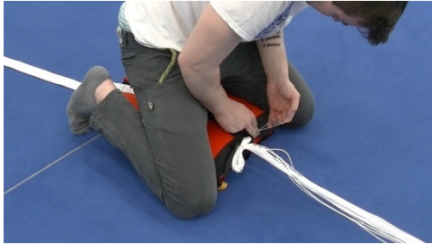
Pic 14.3.3.19 Route left end of the elastic loop through the left grommet
