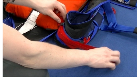
Pic 14.4.1.10 Check correct routing of static line
