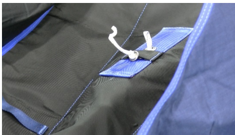
Pic 14.4.1.3 Insert closing loop, stow washer, knot and end of loop under the elastic tape
