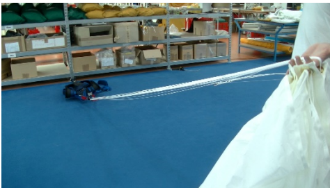
Pic 14.3.2.3 Lift up the canopy, check lines, and hold them under tension
