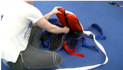
Pic 14.4.1.11 Feed pull up cord (white) through packing cord (red) and pull white cord by red cord through free bag as shown
