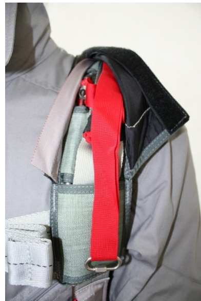
Pic 4.2.2 Static-line; view under the cover
