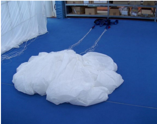
Pic 14.2.3 After inspecting H/C and canopy; place canopy as shown
