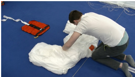
Pic 14.3.3.5 Separate canopy simultaneously, keeping lines under tension using your knees
