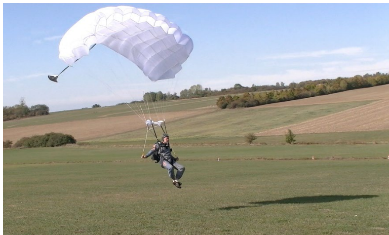
Pic 7.2.3.1 Landing by active flare with steering lines
