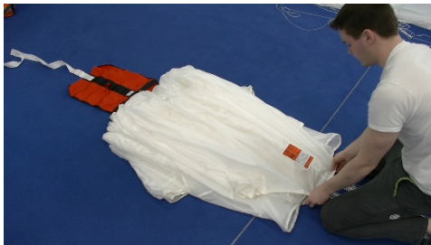
Pic 14.3.3.3 Prepare free bag and pull down center cell
