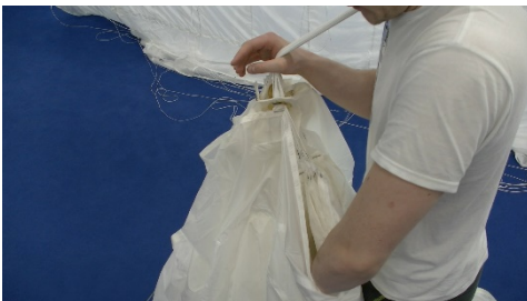
Pic 14.3.2.5 Route lines over the shoulder and start to flake the canopy
