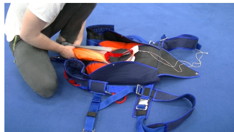
Pic 14.4.3.4 Shape the pilot chute fabric as shown
